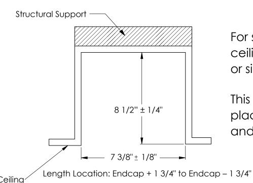
For structural support of the ceiling plate, place a 2' x 4' or similar.
